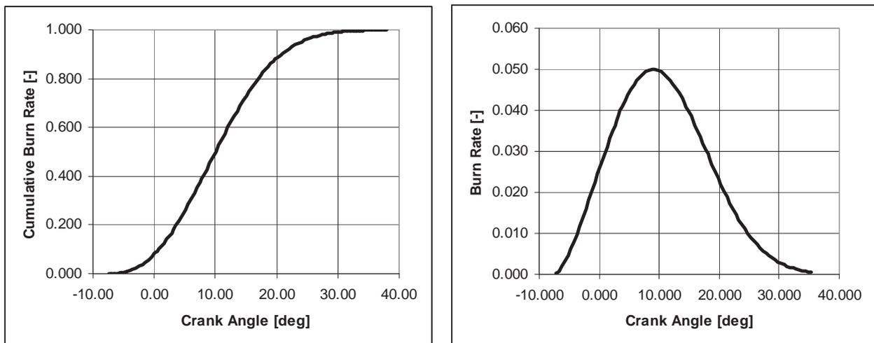
Fig. 4. Cumulative burn rate (left) and burn rate (right) of typical SI engine at full load and 4000 rpm engine speed
