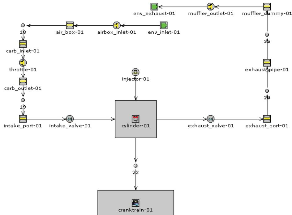
Fig. 2. GT-Power model of simulated single-cylinder engine
