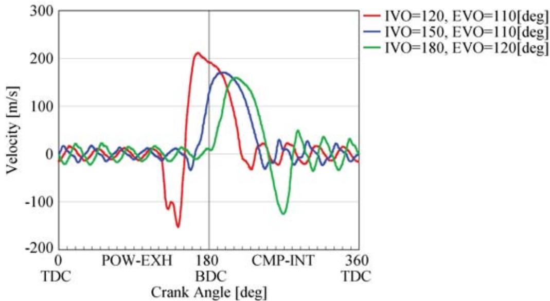
Fig. 7. Air flow velocities through intake port for different valve timing angles
