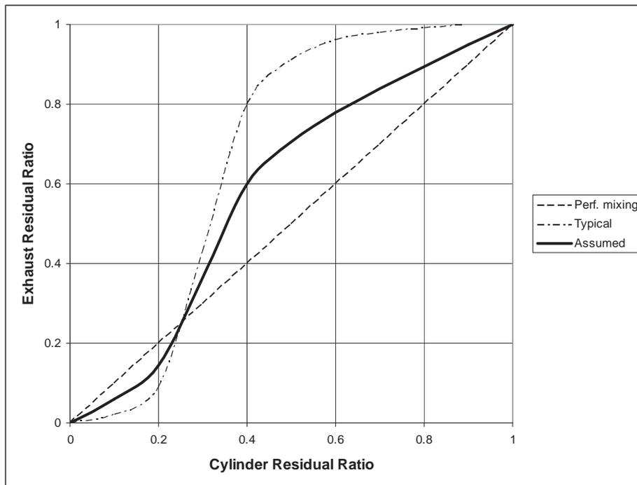
Fig. 3. Scavenging functions: typical two-stroke engine curve, perfect mixing and assumed by authors curves for two-stroke engine with poppet valves
