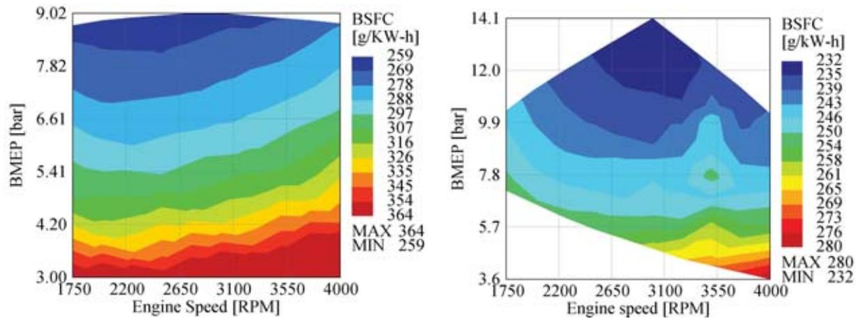
Fig. 8. BSFC map of four-stroke predecessor (left) and two-stroke engine with poppet valves (right)
