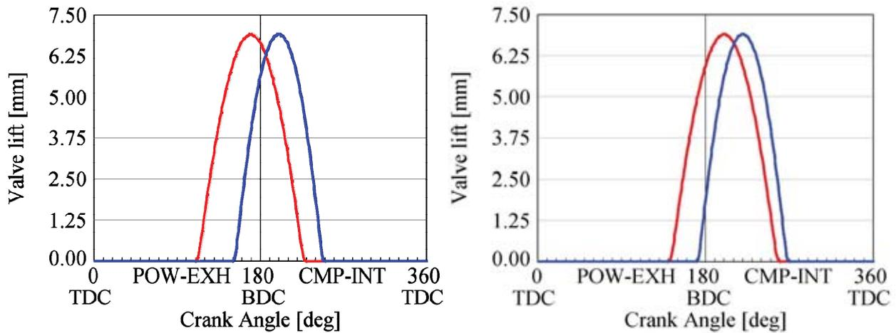
Fig. 5. Intake (blue line) and exhaust (red line) valve lift curves. Left scatter plot presents optimal timing for high BMEP and right for low BSFC
