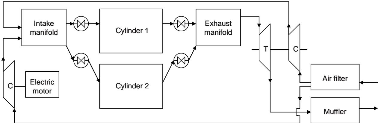
Fig. 1. Flow diagram of new type two-stroke engine with poppet valves
