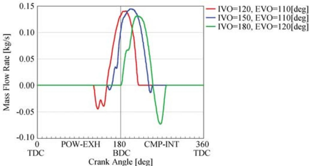
Fig. 6. Mass flow rate through intake valves for different valve timing angles
